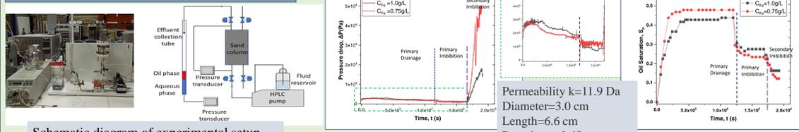
Flow rate at: Primary Drainage 0.4ml/min & Primary/Secondary Imbibition 1ml/min
